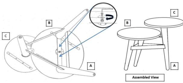
Place the table upside down on a non-marring padded surface. Align & Insert washer (H-2) and Allen screw (H-1) on threaded stud of large top (B) and tighten it with Allen Key (T-1) in clockwise direction as shown above in drawing. Turn the table in upright position. Multi-level accent Table is ready to use.
