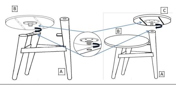
Place the table base (A) on a flat surface and align and install large top (B) on table base (A) as shown in picture above. Rotate large top (B) in clockwise direction until secured with table base (A). Install small top (C) onto table base (A) as shown in picture above. Rotate small top (C) in clockwise direction. Do not over tight large top (B) and small top (C).
